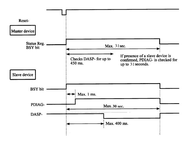
Figure 6.2 Response to hardware reset
